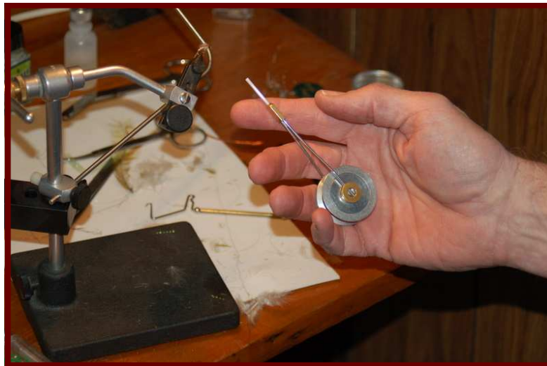
An automatic bobbin works like a window shade - it saves the hassle of rewinding the thread back onto the bobbin
